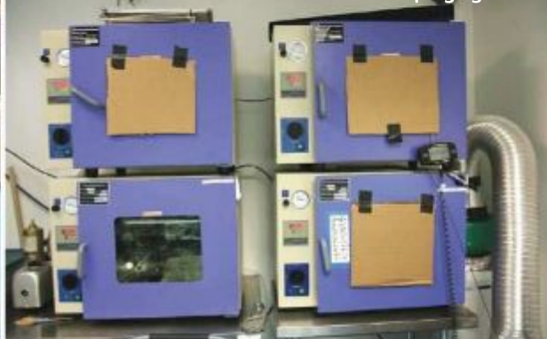
A few of the vacuum ovens Pink House uses for purging.
